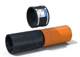
1. Mark both pipes, from the end to be connected, half the width of the coupling, less the required joint gap, which is usually 10mm.
